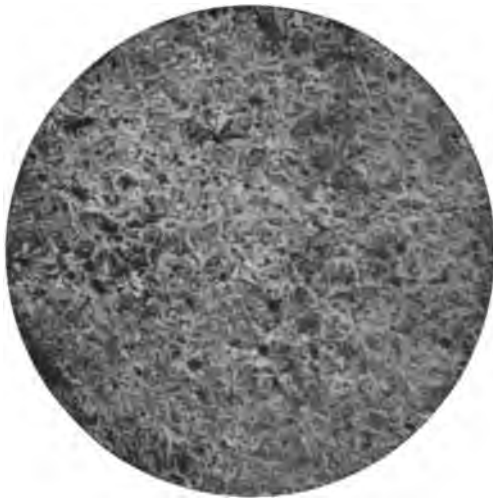
PHOTOMICROGRAPH OF STEM OF TENSILE SPECIMEN C2-G, NO. 7633, CROSS SECTION. 16-INCH BY 18-INCH CARBON STEEL INGOT. MAGNIFICATION 53 DIAMETERS. STEEL HEATED WHITE HOT AND COOLED IN DRY SAND.
